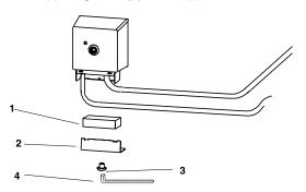
Feed the wires from the transformer through the baseplate. Connect the 1/4" spade terminal to the positive (+) terminal and connect the 3/16" spade terminal to the negative (-) terminal. Terminals are two different sizes and match corresponding terminal clips from transformer.
